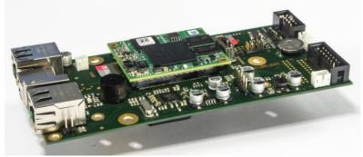
A MPX controller is installed in every Microplex printer ensuring conformity of data acceptance irrespective of the printers installed through out a site
